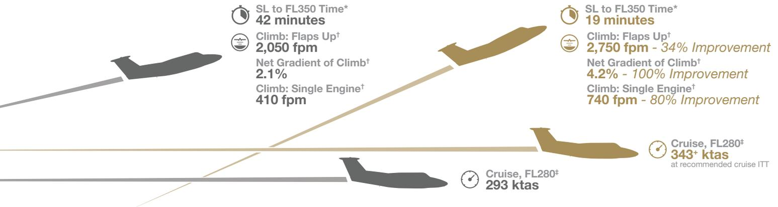
\* ISA +20, Max Gross Weight (14,000lbs) | † Conditions: 30°C, Field Elevation 6000 feet, Max Gross Weight | ‡ ISA +20, Mid Cruise Weight
