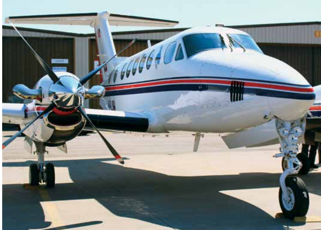
Teton Aviation’s King Air 200 got the Blackhawk engine upgrade, Pratt & Whitney PT6A-61 engines, when it became available in 2008.
