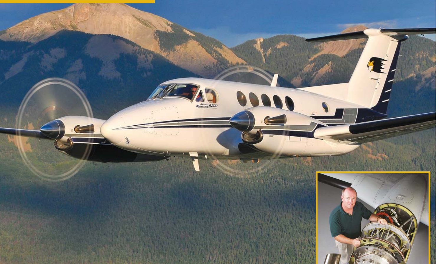
A BLACKHAWK CONVERTED KING AIR B200, AND (INSET) JIM ALLMON WITH A PRATT & WHITNEY CANADA PT6A-135A ENGINE
